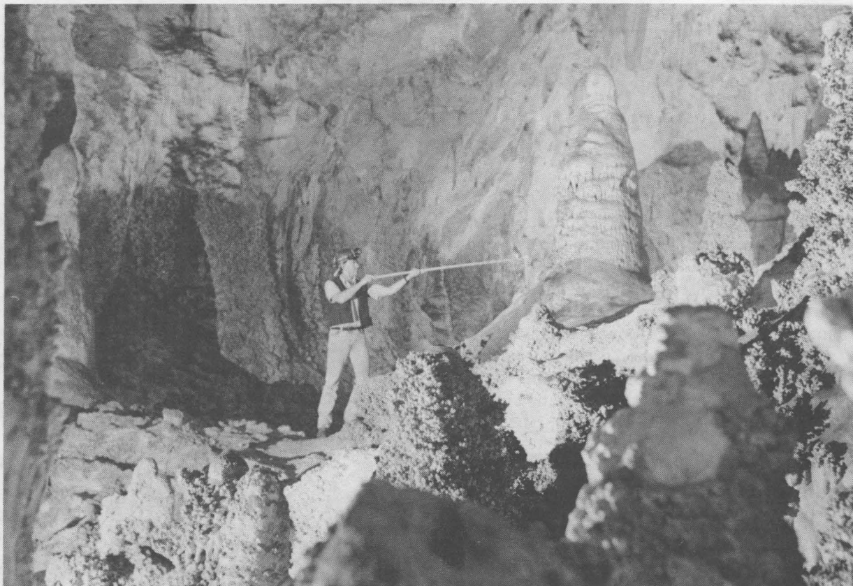
AT SOME DRIP SITES where it is not possible to set up a stand, such as this one on the side of a stalagmite near the Hall of Giants, Steve Lambert (6233) collects water samples by attaching a funnel and cylinder to a long wooden pole.
